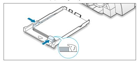
6. Slide the paper input tray in. If the paper output tray was up, flip it back down.
